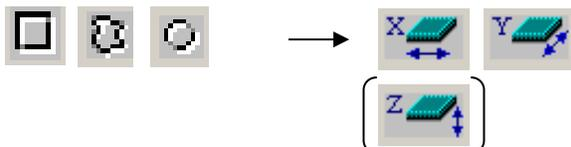
For area mapping X and Y dimensions need to be defined. For volume, define the Z dimension as well.
