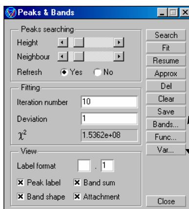
Opens a new window displaying the results of the band fit for baselines and peaks. (p=position, w=full width half max., a=amplitude or max. intensity, g=Gaussian contribution, s=integrated area)
