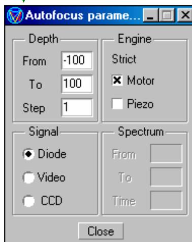
Force the software to use either the Z motor or the piezo for autofocussing.
