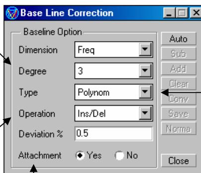
Type of baseline approximation: either *polynomial* (data points lie on a polynomial curve), or *line segment* (data points joined by straight lines)
