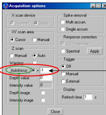
Offset (in  $\mu\text{m}$ ) to be applied to the calculated focus position.
