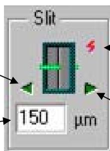
Reinitialise the slit – sends the slit to a known reference point, and then back to the position displayed in the box.
