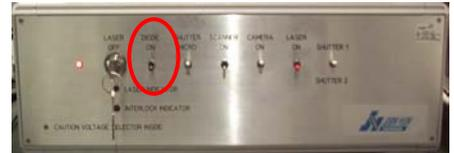
6. You should now see the red diode spot on the camera image. Adjust the microscope focus to bring the spot to a tight focus.
