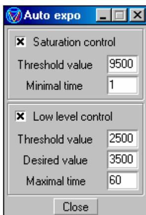
**Saturation control** - sets the upper limit for acquisition eg. 9,500 counts. If this limit is reached it will calculate the acquisition time required to bring the spectrum below this threshold. A minimum time value can be set so that the system does not try to continually adjust this ad-infinitum.
