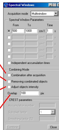
Note that individual windows can also be manually combined after acquisition simply by clicking on the COMBINE button. The *Remove combined objects* and *Adjust objects intensity* check boxes will still function.
