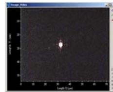
7. Close the confocal hole down to between 50  $\mu\text{m}$  and 100  $\mu\text{m}$  (ensuring you can still see the diode spot on the camera image). Adjust the focus again.
