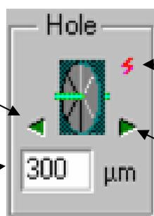
Reinitialise the hole – sends the hole to a known reference point, and then back to the position displayed in the box.
